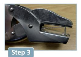
Manipulate the pliers with a quick CLOSURE SQUEEZE without any pull towards the operator's body until the tag is clinched.
