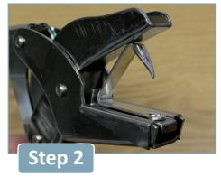
Insert the tag into the pliers and seat into the indent. Ensure the tag is seated correctly against the jaws.
