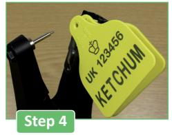
Once the tag is applied, release the handle, to allow the male part of the applicator to retract.
