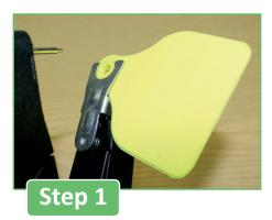
Locate the female part under the correct clip. The back of the female tag slots into the applicator.
