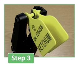
Line up the male and female parts of the tag and squeeze the applicator to clip together.
