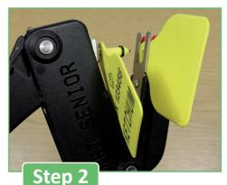
Locate the male part of the tag into the applicator pin and seat correctly.
